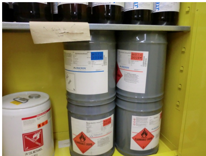
Figure 2. Containers with Insufficient Clearance
