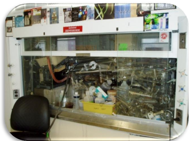
Image 1: Over-crowded fume hood with no working space and no ventilation.
