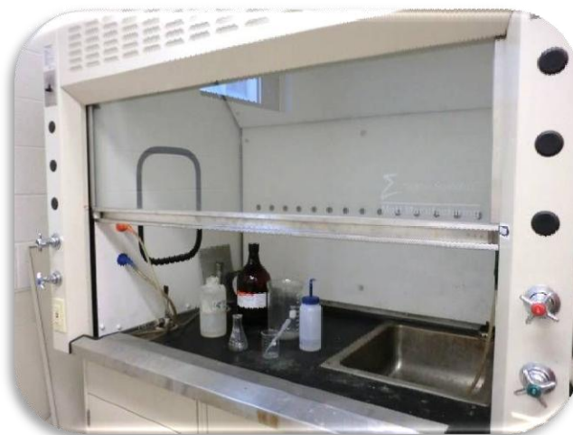
Image 2: Good fume hood practice with plenty of work space and good ventilation.
