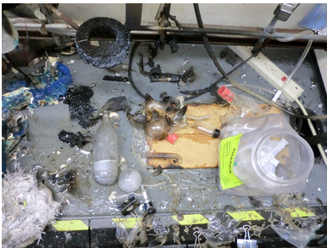
Figure 1: Contents of Fume Hood after Explosion
