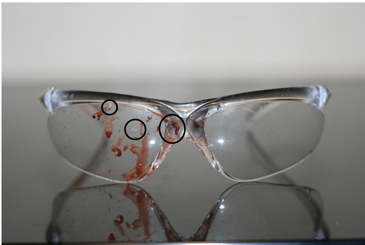
Figure 2: Safety Glasses Worn by Researcher. Some of the areas of impact have been highlighted.
