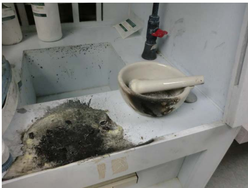
Fume Hood after Fire
