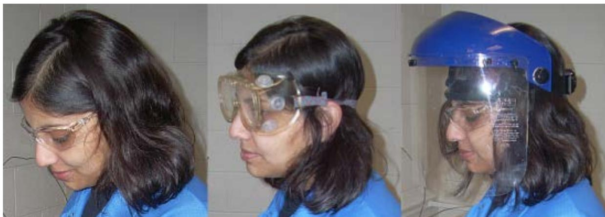
**Left: Safety Glasses;    Center: Chemical Splash Goggles;    Right: Face Shield over Safety Glasses.**
