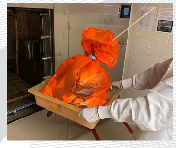
4. When removing sterile, hot items, use **thermal gloves**.
