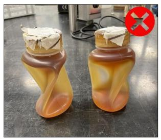
**Autoclave Loading: A**. Ensure that bags are loosely closed. Use a cart for heavy items and use a secondary container. Always wear proper PPE and closed toe shoes when handling biohazardous waste, and do not carry bags from the bottom. **B**. Caps must be loosened for any bottles containing liquid and add 1-2 cm of water to the secondary container. Do not overfill bottles.
