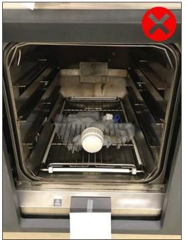
**Autoclavable Materials:** Materials loaded into an autoclave must be made to withstand autoclaving. Autoclaving materials that are not marketed as such will result in damage to the item as well as the autoclave.
